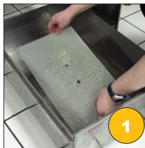
Place clean filter screen on bottom of clean filter pan
