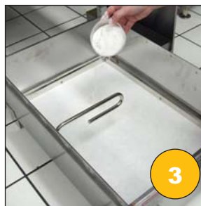
Place filter hold-down on top of filter paper and spread Bro-Clean filtering compound on top of paper – 1 cup for 1600, 2 cups for 1800, 3 cups for 2400.
